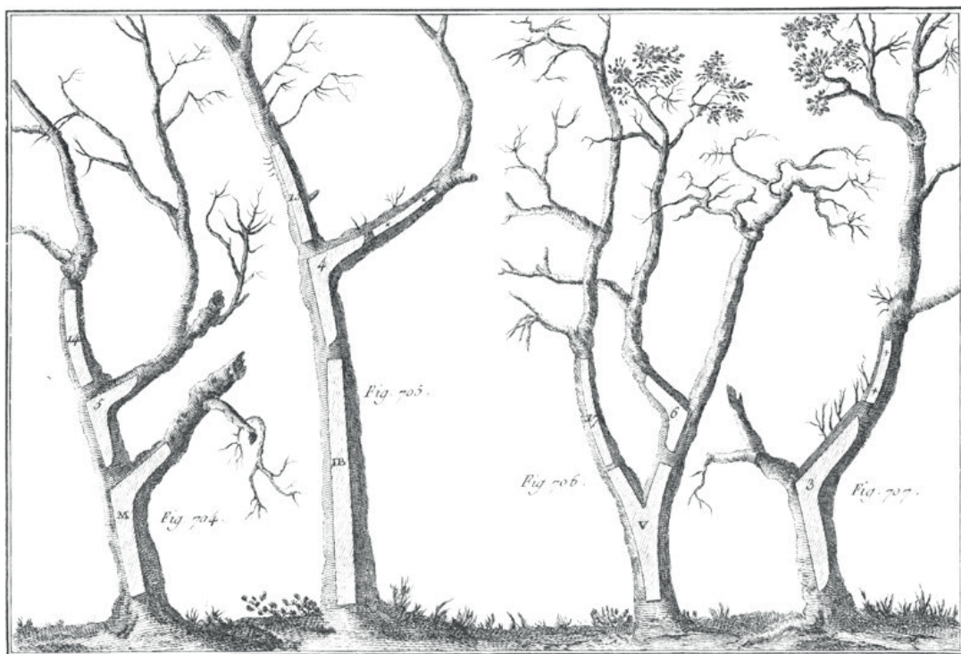
Courtieu, natural deformations for naval construction, extrait of Encyclopédie méthodique marine, p. 103: the influence of (Venitian) naval timber construction is evident on the Pontelarisma technique, see next photos of angular reinforcements.
