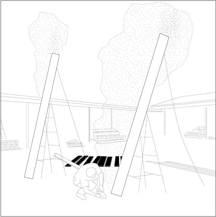
Charring wood (Yakisugi technique) to increase the resistance to insects, mould and decay
