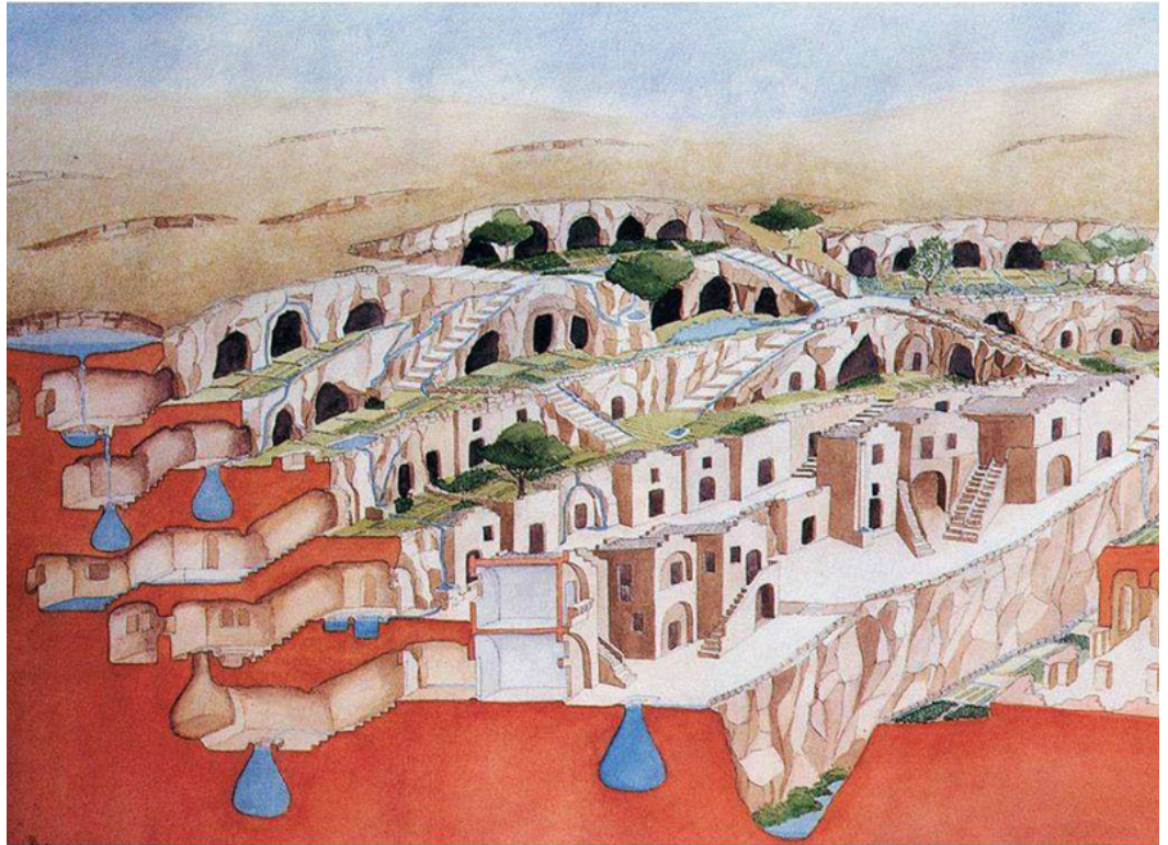
Fig. 84 Sketch showing a idealized section of a settlement along a valley cliff at Matera
