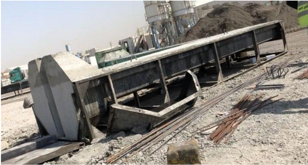
Figure 54 concrete T wall mold, 2021 Photograph by the Kali Rubaii
