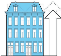
FACADE STRETCHED TO FIT NEW VOLUME
