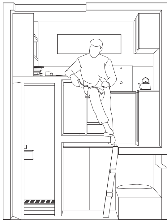
fig 16. A perspective section of Absalon's Cell No. 5 , illustrating the separation of functions on different levels, accessed by a ladder. Drawn by the author.
