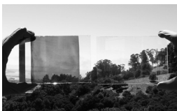
Electrochromic glass able to change opacity
