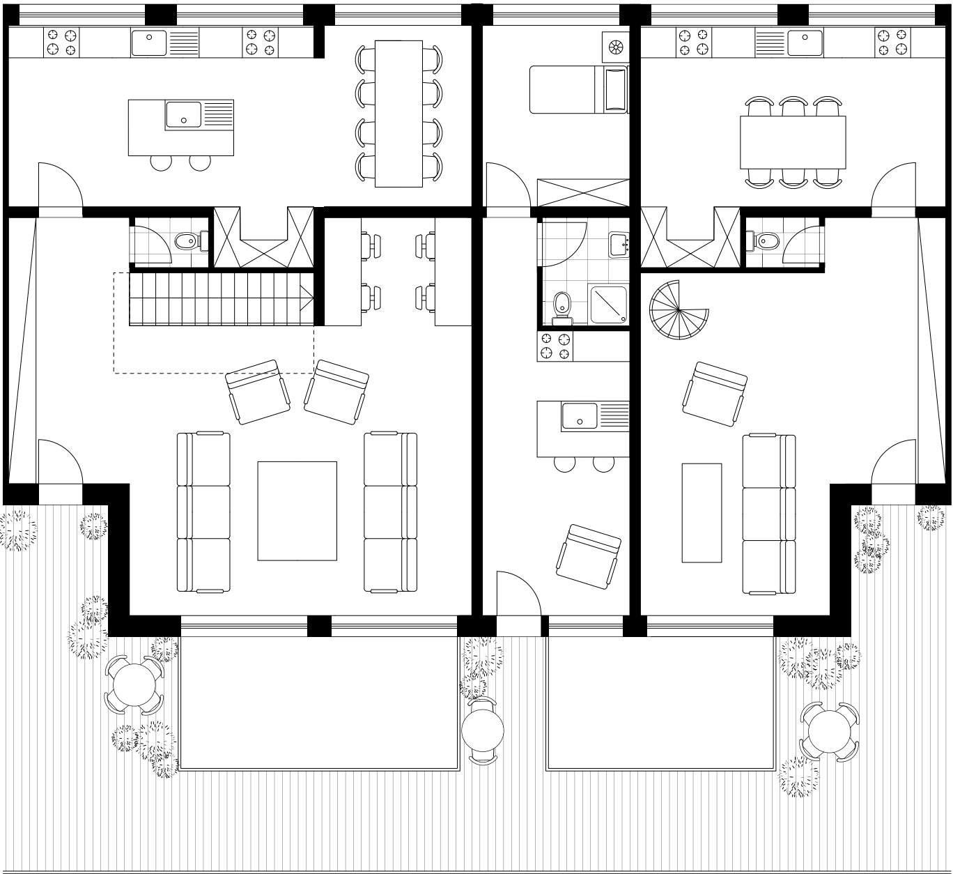
Plan duplex 1er étage (246 m²)/simplex (31 m²)/duplex (138 m²)1:100
