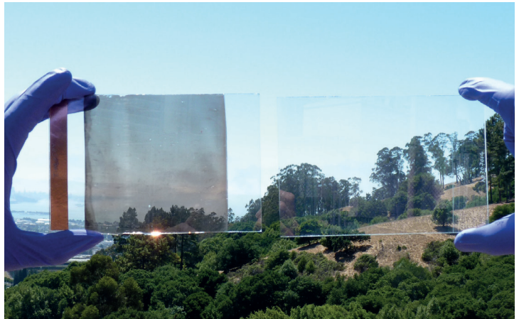
Electrochromic glass able to change opacit
