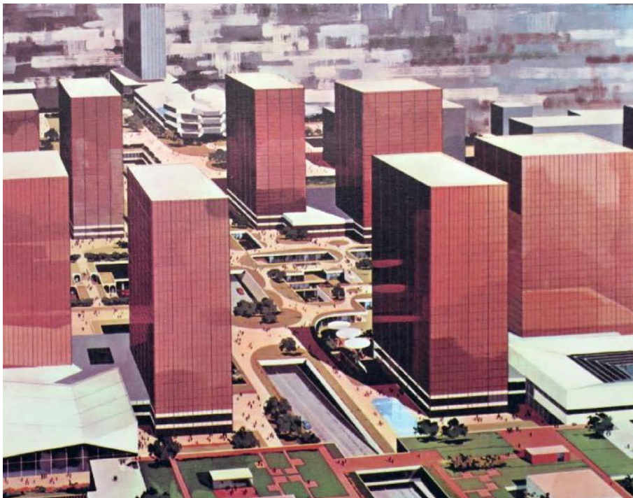
Figure 5: Drawings of the pedestrian walkways, on the plinths and in between of the WTC Towers, that frees up the traffic below. De Beule, 2017: 357.
