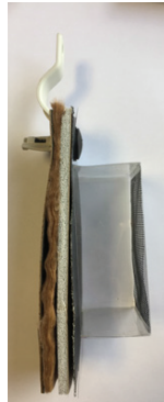
Better Shelter - polyolefin (8mm) - UV protection film
