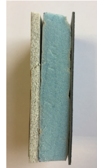
Add. Insulation #2 - polyolefin (8 mm) - UV protection film - expanded polystyrene (20 mm) - Altro Xpresslay (2 mm)
