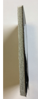
Step 2 - polyolefin (8 mm) - UV protection film - tarpaulin - PET sheet
