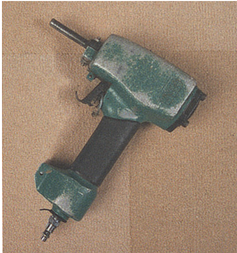
Figure 24. Photography and illustration by the ReUse People, Reconnx Nail Kicker pneumatic nail remover and instructions
